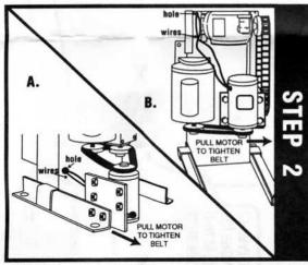
BOLT DC MOTOR TO PLATE OF STEP 1A OR 1B. PUT NEW BELT IN PLACE AROUND PULLEYS. MAKE SURE PULLEYS ARE IN LINE. PULL MOTOR TO TIGHTEN BELT, THEN FINISH TIGHTENING BOLTS. PUT TWO WIRES FROM NEW MOTOR THROUGH APPROPRIATE HOLE IN CHASSIS AS SHOWN.
