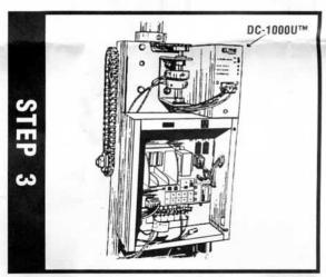
PLACE DC-1000U™ UNIT ON TOP OF MAIN CONTROL BOX AND INSTALL TWO WIRES FROM BACK OF DC-1000U™ TO TWO WIRES FROM 12V MOTOR, USING WIRE NUTS PROVIDED. (CROSSING WIRES WILL CHANGE THE DIRECTION THE DC-1000U™ WILL OPEN.)
