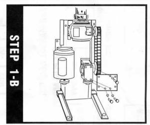
REMOVE EXISTING BELT. MOUNT NEW PLATE ON LOWER GEARBOX. BOLT IN PLACE (AS SHOWN) WITH BOLTS PROVIDED.
