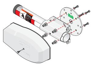
Wire Harness Note: Unplug wire harness inside operator and remove wire guard from operator housing BEFORE unbolting arm from hub when necessary.
