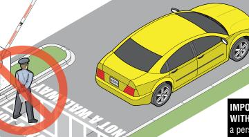
**IMPORTANT:** A barrier gate operator installed **WITHOUT** any safety sensors **CANNOT** sense a person under the raised arm and can strike them while the arm is lowering.
