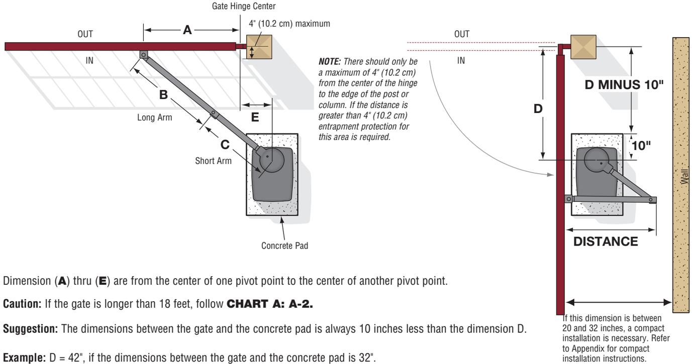
Dimension (A) thru (E) are from the center of one pivot point to the center of another pivot point.
