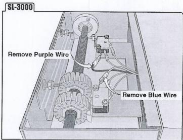
The blue and purple wires are NOT used on the limit switches with the OmniControl™ board. Reconnect power to operator after installation is complete.
