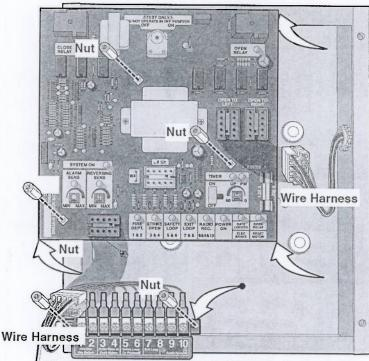
Disconnect power to operator. Disconnect the 2 wire harnesses and remove the old board by removing the 3 nuts. Remove the terminal connection strip by removing the 2 nuts. Reverse this process to install the OmniControl™ board.
