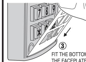
③ FIT THE BOTTOM TAB OF THE FACEPLATE INTO THE SLOT ON THE KEYPAD
