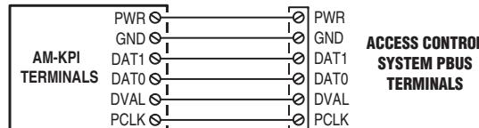
EACH REMOTE DEVICE MUST BE SET TO A UNIQUE NUMBER FROM 1 TO 6
