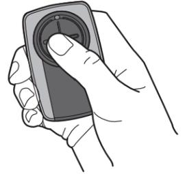
The LED on the Universal Remote Control **MUST** stop blinking between each press of the button. The code is accepted when a click or beep is heard, a light blinks, or the door/gate activates.
