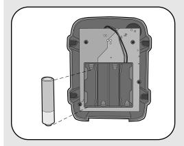
Install 4 AA Alkaline batteries (not provided). (Lithium batteries recommended for colder environments.) Keypad will beep.
